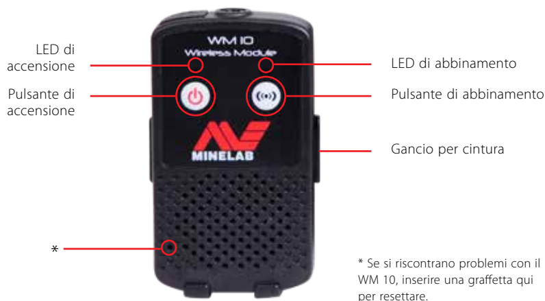
Figura 35 – Modulo audio wireless (WM 10)
